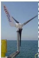
A wind turbine (wind generator) is a system that converts the kinetic energy of the wind into electricity. The principal of operation is similar to a hydroelectric generator. The main difference is the medium that is being utilized, running water for the first and blowing wind for the latter.
