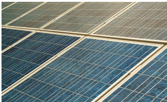
picture 4 – close-up of the test modules (modules above with normal solar glass and below modules with Sunarc anti-reflex coating)
